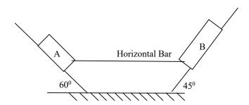
Two cylindes A & B of diameters 60 mm and 30 mm weighing 80 KN and 20 KN respectively are placed in a channel. Find out reactions at all the contact points.
